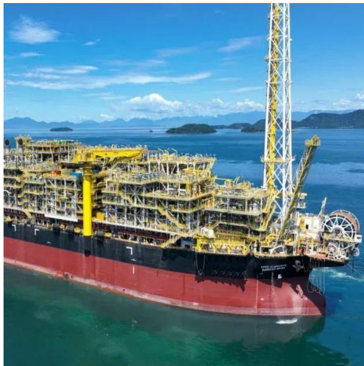
(b) Prediction of heave motion for FPSOs: FPSOs (Floating Production Storage and Offloading) are large, semi-submerged ships used for processing, storing, and offloading hydrocarbons from subsea wells. Due to floating nature, FPSO are highly susceptible to heave motion, which are the vertical oscillation caused by wave action. Accurate prediction of this motion is essential for ensuring operational safety, equipment integrity, and smooth production processes.
