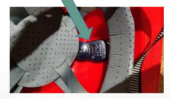
When people go to the electrical construction/maintenance site to work, an induction detection module is installed on the casing that matches the pressure sensor. If an abnormality is detected, a buzzer is installed inside the casing that matches the induction detection module to warn people and avoid physical injury.
