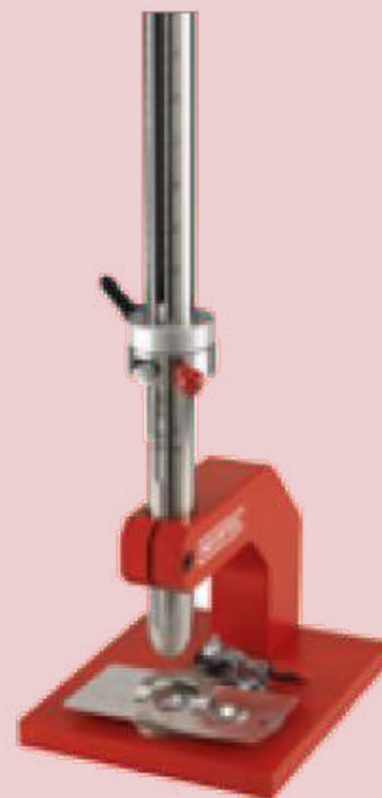
Device for measuring the resistance of coatings to impact according to ISO 6272
