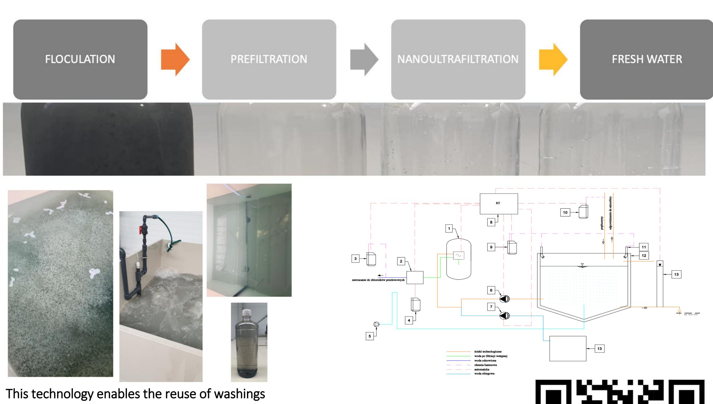
This technology enables the reuse of washings from the filters of spa pools up to 96%, which significantly reduces the need for brine water, reduces the costs associated with its heating and sewage disposal. The installation is characterized by the retention of solid suspensions, colloids, bacteria, viruses, but not the removal of salts dissolved in water, which is especially important so that the composition and concentration of cations and medicinal anions do not change.
